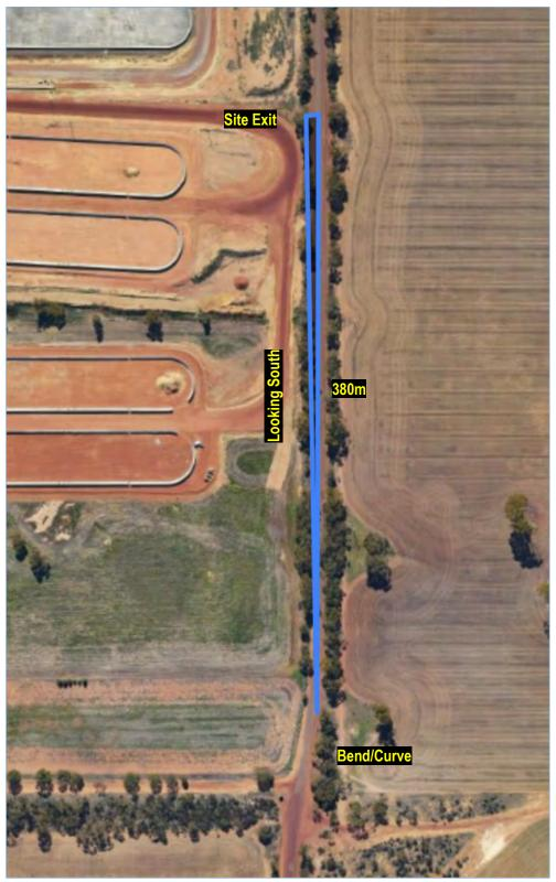
Figure 8: Sight distance check - New Site Exit - South
