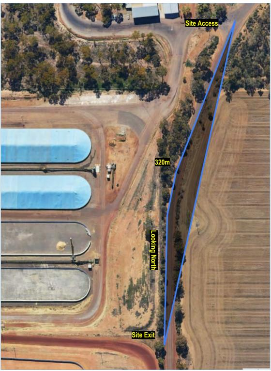
Figure 9: Sight distance check - New Site Exit - North
