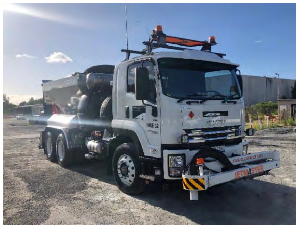
Patching Boom fully retracted for travel.
