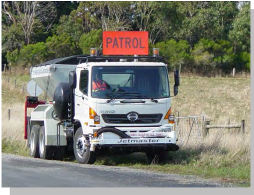
Jetmaster® boom fully retracted and stowed for safe travel between repair jobs.
