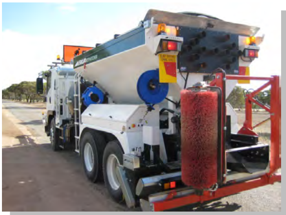
6m 3 AUSROAD Jetmaster ® road maintenance unit with Jetmaster ® remote control boom, owned & operated by District Council of Copper Coast, SA.
